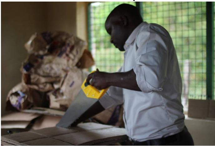
An orthotist cuts out a chair from board, based on a child's measurements.
